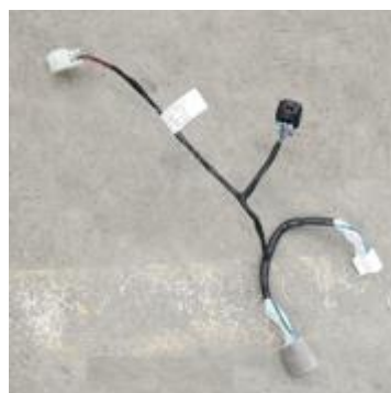
Patch loom for connection behind LH front floor kick panel
